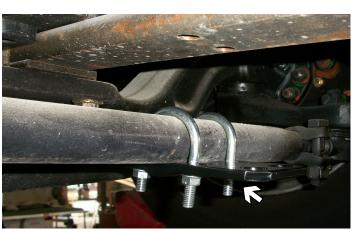
4. Install Tie Rod Bracket (Item 3) on the passenger's side tie rod using the appropriate U-Bolts for your application (Item 4 - 1 7/8" or 2"), according to drawing on page 3. DO NOT TIGHTEN. Tie Rod Bracket may be rotated or flipped to insure Steering Control (Item 1) remains parallel to the ground.
