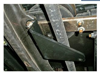
Slide the Anchor Bracket (Item 2) on the axle on the driver's side. The plate offsets toward the center of the vehicle. Reinstall the existing washers and nuts and tighten to manufacturers specifications. Bracket must clear tie rod at least 1/4".
