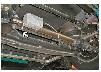
Install solenoid end of the TruCenter (Item 1) to the top side of the Anchor Bracket (Item 3) with 3 1/2" bolt, 3/4" flat washers and 1.59 flange nut (Items 5, 6 and 9), according to drawing on page 3.
