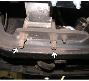
2. Remove two nuts from the driver's side axle pad.
